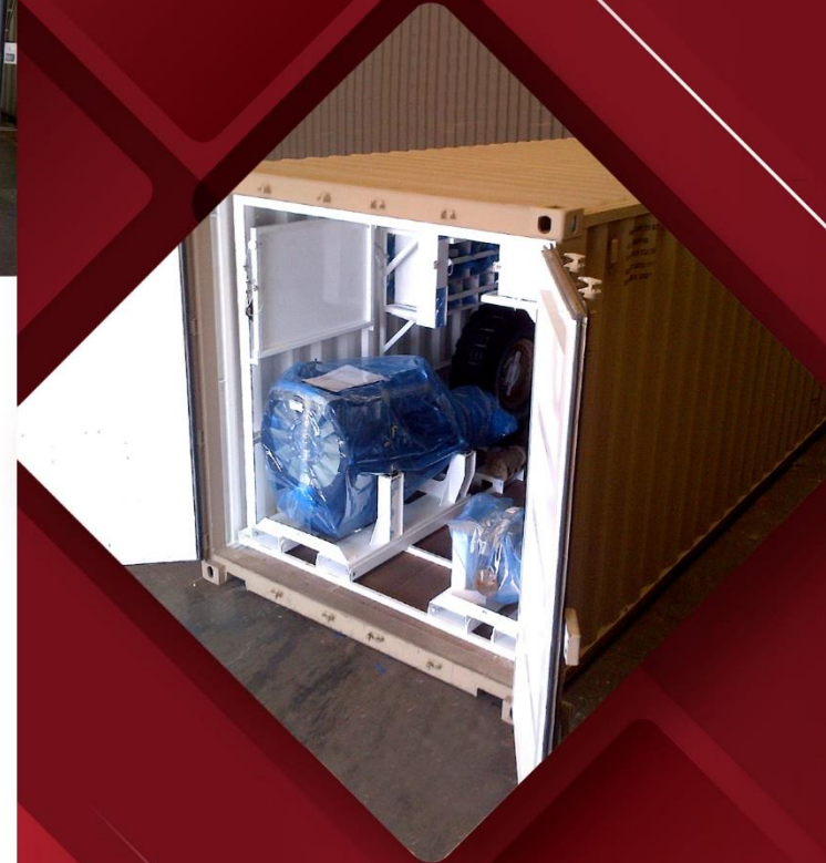
Inside left view with fold down work bench above the Engine assembly in the stowed position and various spare parts and bins.
