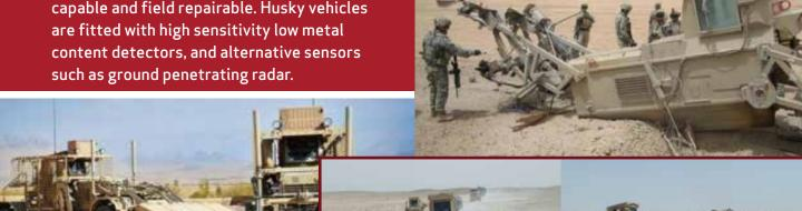
The Husky is a versatile sensor platform that can detect, mark and interrogate land mines and IED threats depending on the equipment fitted to the vehicle. In the event of a detonation, the components have been engineered in a unique configuration that breaks apart in a predictable manner. This facilitates fast in-field repairs, while any damage to the system can usually be repaired in the field, increasing uptime and system availability.
